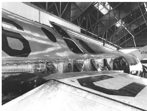
**Figure 26. NF-104A Hydrogen Peroxide Damage**
