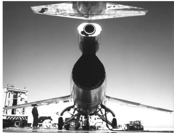
Figure 4. NF-104A Turbojet and Rocket Motor
